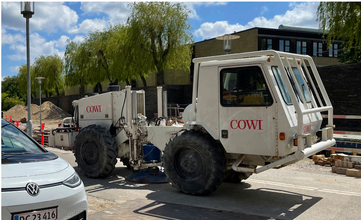
To assess the impact of the upcoming light rail on DTU Nanolab, DTU and Rambøll used a "shaker" to conduct seismic measurements around Ørsted's Plads. The shaker simulates the vibrations caused by passing light rail trains. It was kindly loaned to Rambøll by Cowi. Photo: DTU
