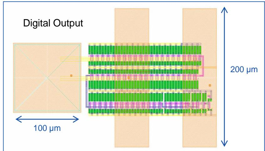
Drive off chip capacitance=20 pF at  $t_{\text{rise}} \sim 1 \text{ ns}$
