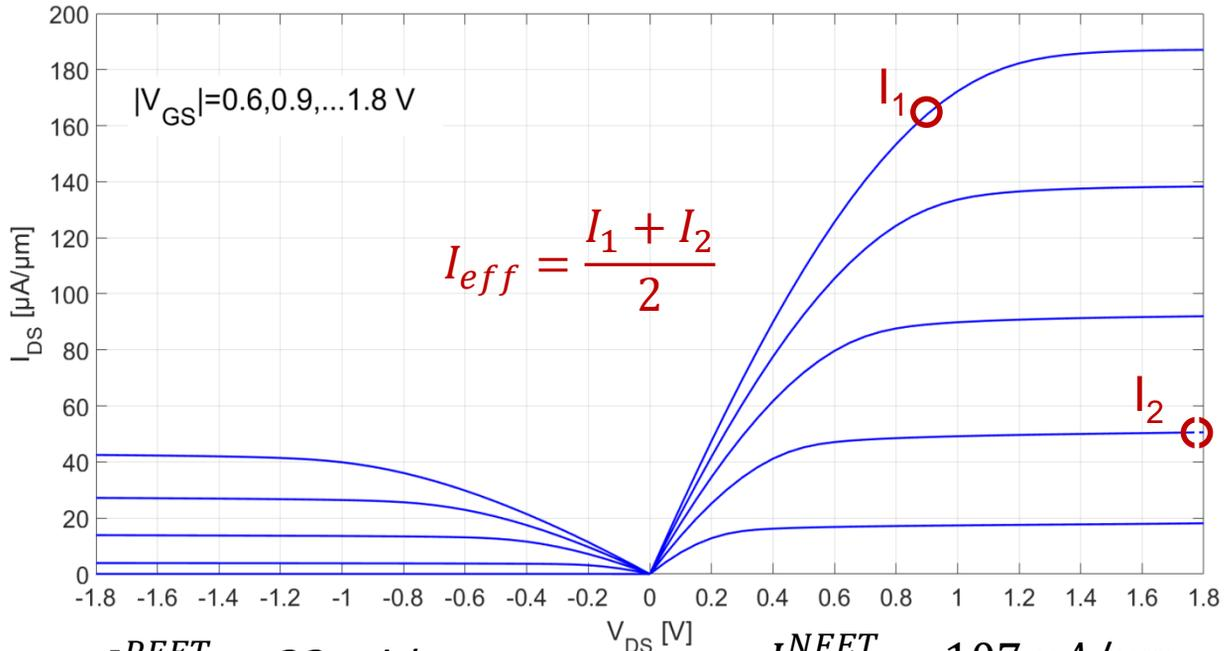
$$I_{eff}^{PFET} = 22 \mu\text{A}/\mu\text{m}$$
