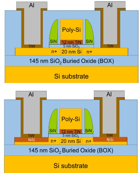
All devices have TiN deposited by PVD (magnetron sputtering).
