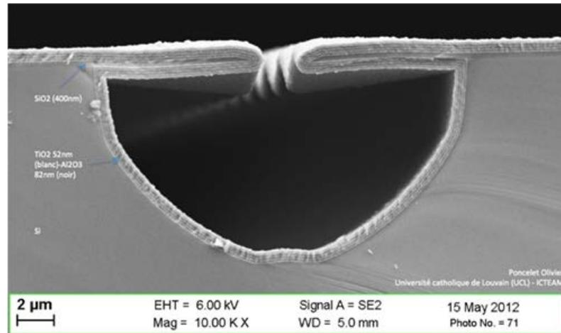
**Al<sub>2</sub>O<sub>3</sub> and TiO<sub>2</sub> layers deposited in a 3D cavity**
