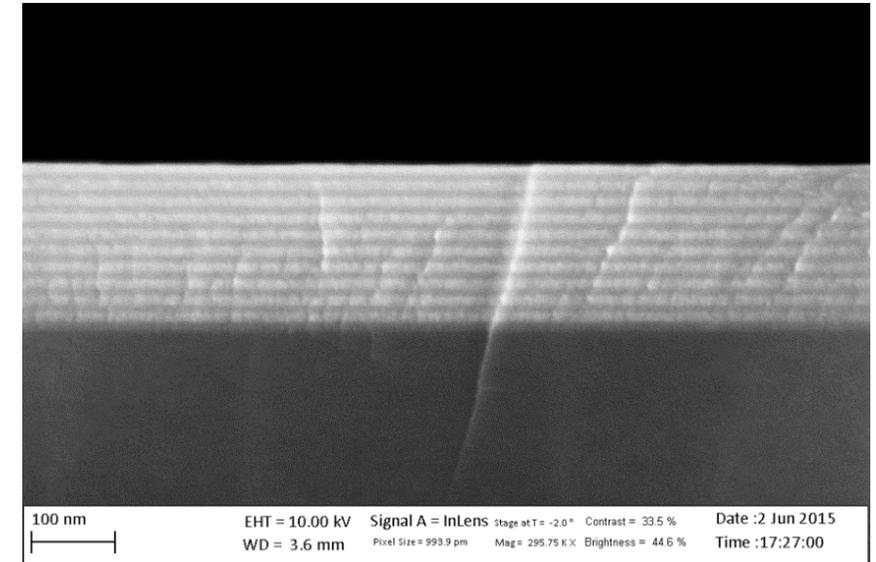
**Si sample with multilayers of Al<sub>2</sub>O<sub>3</sub> and TiO<sub>2</sub>**
