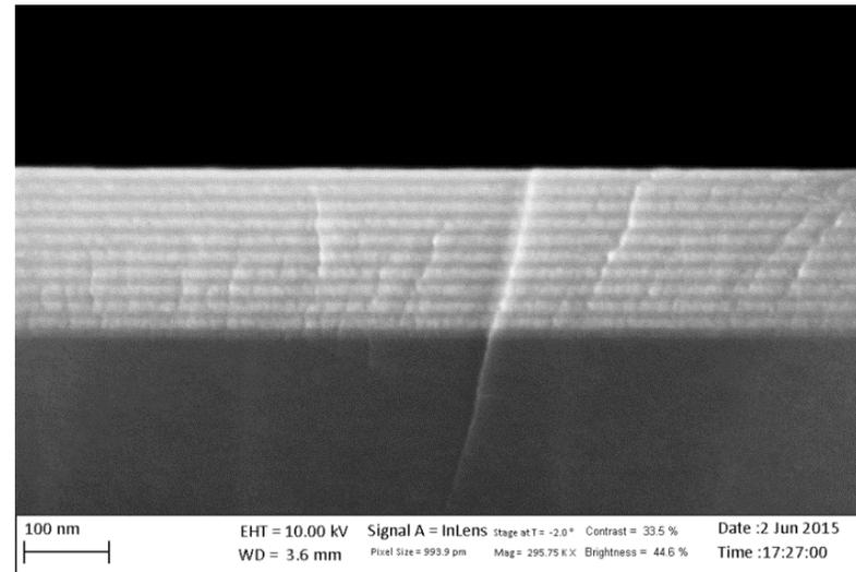
**Si sample with multilayers of  $\text{Al}_2\text{O}_3$  and  $\text{TiO}_2$**
