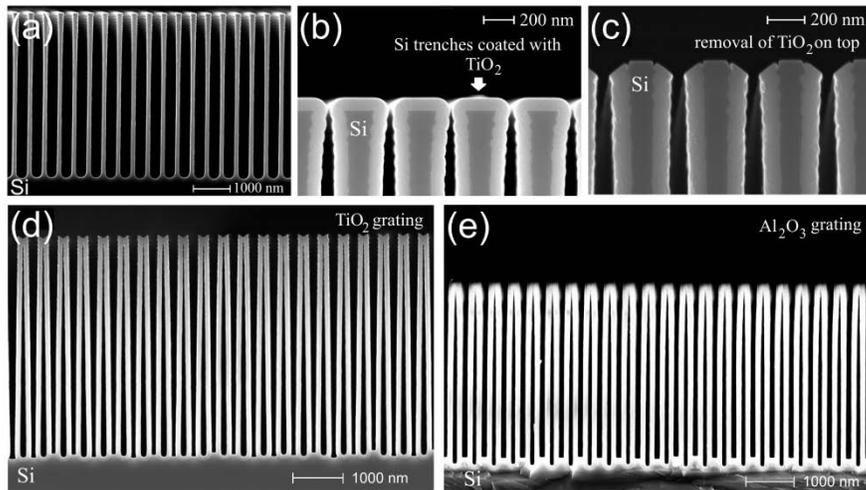
(a) Fabricated silicon trenches. (b) TiO<sub>2</sub> ALD coating of trenches. (c) Selective opening of the top parts of the gratings. (d) Fabricated TiO<sub>2</sub> and (e) Al<sub>2</sub>O<sub>3</sub> gratings.
