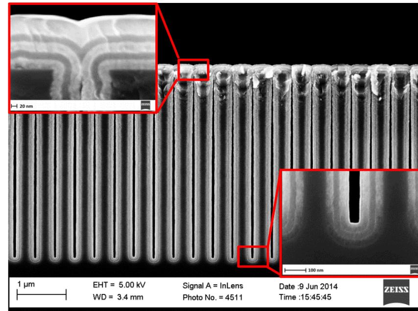
**Al<sub>2</sub>O<sub>3</sub> and TiO<sub>2</sub> layers deposited on high aspect ratio trenches**
