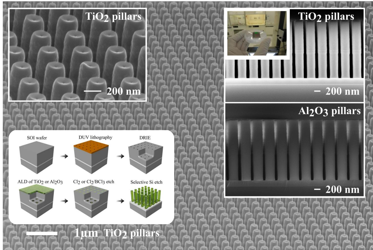
Fabrication of TiO<sub>2</sub> and Al<sub>2</sub>O<sub>3</sub> pillars. The concept and final realization.
