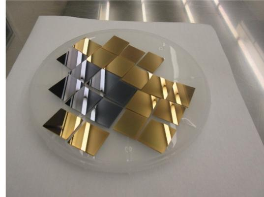
Si trench template covered with TiN before and after annealing at 900 °C. Silver and gold colored chips, respectively.
