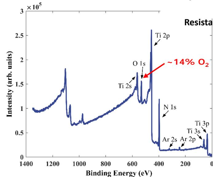
XPS measurement of TiN deposited at 500 °C
