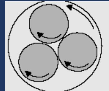
AIXTRON 200/4 – Horizontal cold-wall reactor, 3x2-inch configuration with gas-foil main and satellite rotation
